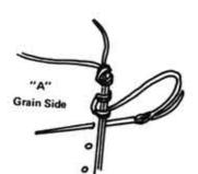
Step 8. Using excess thread from heel, sew lower part of heel together using the running stitch. Align holes and edges for horizontal seam. Insert thread through first 2 holes as indicated. Use running stitch. As you sew to the center, insert thread through last hole of vertical seam and back up through hole on other side of vertical seam. An awl may be used to help align holes.
