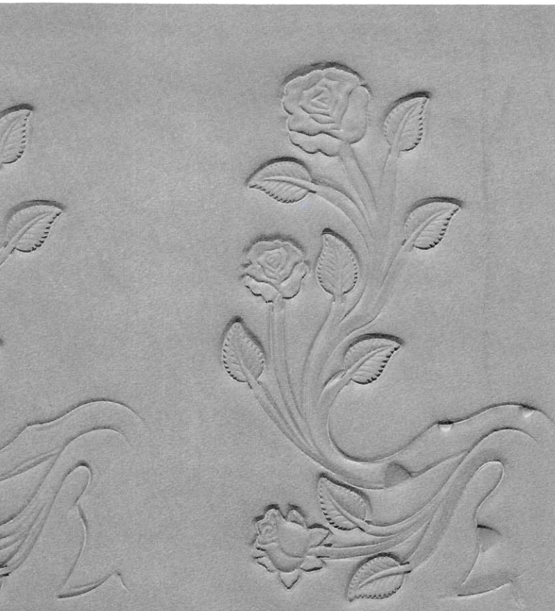
Step 4 – Bevel stems, on inside of stem lines using Crafftool #F891 and F895.
