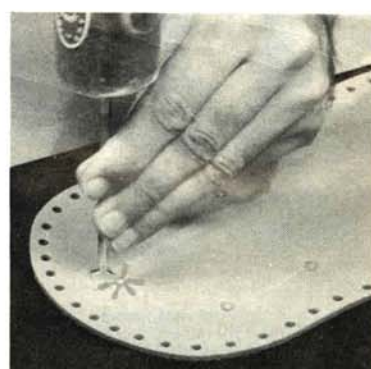
Step 5: Stamp four more impressions with Craftool P368 as shown. Space them half way between the previous impressions. Stamp two impressions between each previous impression with Craftool P368.
