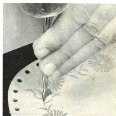
Step 5: Stamp four more impressions with Craftool P368 as shown. Space them half way between the previous impressions. Stamp two impressions between each previous impression with Craftool P368.
