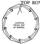
Begin lacing from inside the FUN BARREL, Lace through hole #1 and #2, which overlaps #1. Return the lace to the inside of the barrel through holes #3 and #4, which over-
