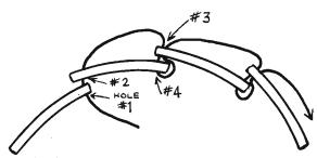
Bring lace around side of Stave B and in between stave B and C. Pull lacing through the hole #3 which is on Stave C. Lacing should now be on outside of the barrel. Return lacing to inside of barrel through holes #5 and #6. Repeat this process until all ten staves are laced securely together. After lacing has been returned to the inside of the barrel for the last time, the loose end should be tied to the other loose end of the lace. Lacing on outside of barrel should appear as illustrated.
