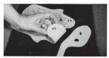
Step 5. Set the Durable Dot Snaps with the Durable Dot Snap Setter and Anvil. (See Durable Dot Snap Setting Instructions.) Set the studs and eyelets on "A" and the buttons and sockets on "B" as shown.
