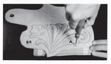
Step 7. Use cutting pattern to locate stitching holes. Stab the holes through the leather on parts "A" and "B" with a stitching awl. Use a protective pad such as several layers of corrugated board when stabbling the holes.
