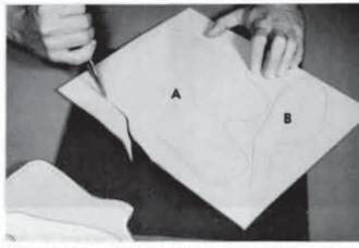
Step 1. Use the cutting patterns to cut out the holster part "A" and strap part "B" for the holster that you wish to make. Place the cutting patterns on the grain side of the leather with a placement that will allow you to cut out both parts. Trace over the cutting lines with a stylus or ballpoint pen. A light impression will be made in the leather for you to use as a guide. Use a sharp knife to cut along the lines.
