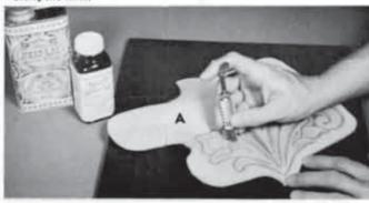
Step 3. Tool, dye and apply leather finish to your holster, if you prefer, a very durable and attractive holster can be made by applying Neatsfoot Oll. Apply light coats until you achieve the shade desired. You can experiment with the scrap pieces.
