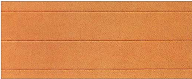
1. Scribe guidelines lightly with Wing Divider #3607-00.
