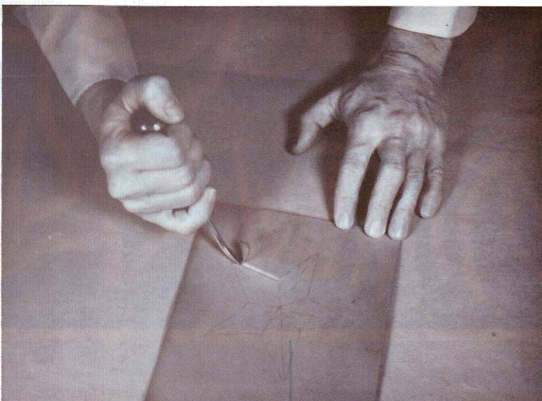
Step 2. Cut design into leather, holding gouge as shown and gouge about \frac{1}{2} the thickness of leather. (When gouging straight lines you may use a "straight edge" of some kind to guide gouging tools.) When cut is completed, lift gouge from leather leaving "plug" attached to leather.
