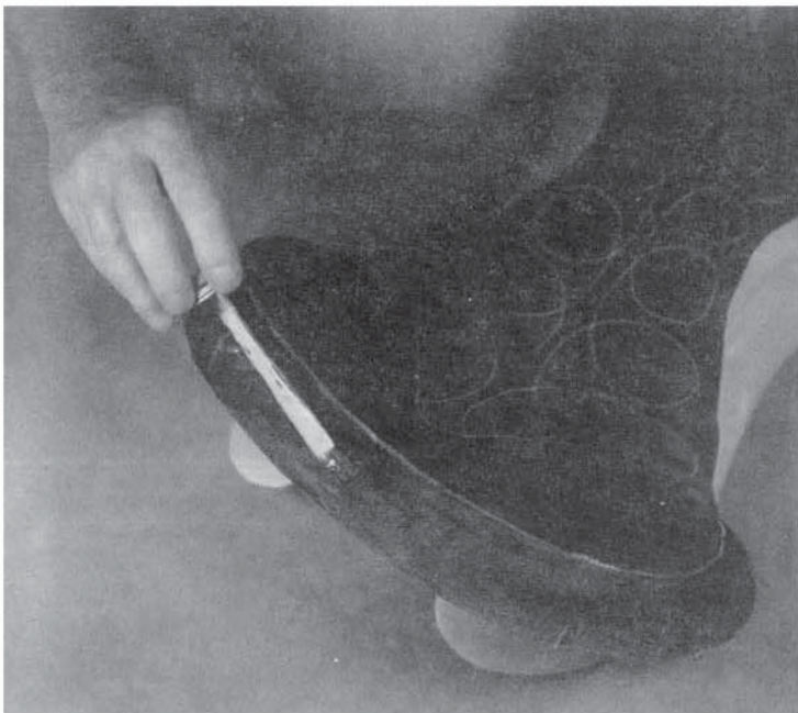
STEP 23. Apply craftsman cement to suede seat cover in area over cantle filler.
