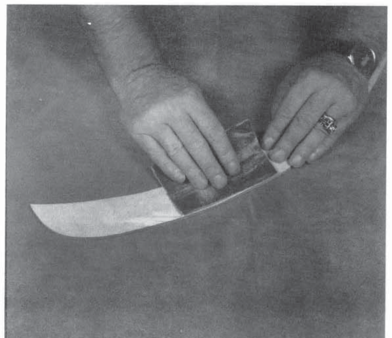
STEP 8. Rough-up both sides of cantele filler with sandpaper.
