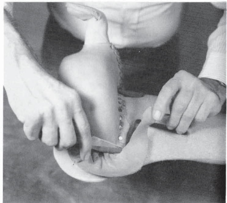
STEP 11. Trim away excess leather, as shown.
