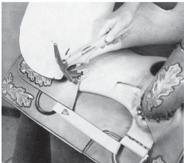
STEP 8. Secure both sides of back jockeys assembly to tree with small tacks, as shown.
