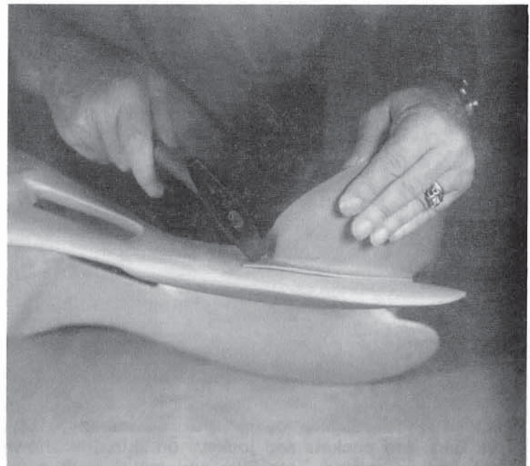
STEP 4. Dampen cover thoroughly then form over back of cantele on tree. Secure temporarily at corners with 2 small tacks.
