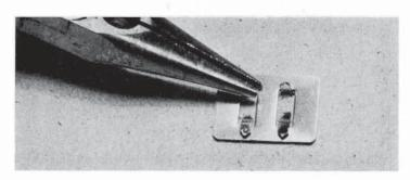
STEP 2. To install twist clasp in bag front, align tracing pattern over bag front and mark position of bag clasp holes with an awl. Remove pattern and force awl through the leather at each mark or punch holes at each mark with No. 1 punch. From carved, smooth side of bag front insert prongs of twist clasp through holes. On rough side of bag front, place twist clasp back plate over prongs and with pliers or hammer bend prongs outward over back plate. Prongs should be flat as possible.
