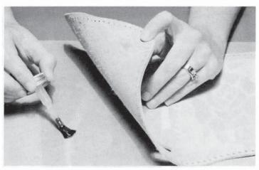
STEP 1. To prevent leather from stretching while carving and stamping the design, cement leather to cardborad or heavy wrapping paper. Apply a light coat of rubber cement to rough side of leather and to cardboard. Allow cement to dry and adhere leather to cardboard and you are ready to carve and stamp your design.
