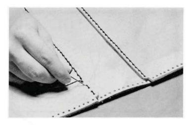
STEP 8. Using instructions in Step 3, cement lining piece with pocket to bag back. Align holes in bag back over holes in other side of bottom piece, smooth sides up. Stitch together using instructions in Step 7.
