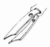
STEP 1. Insert one end of leather lace through eye of zipper "pull" fold in half and laign holes.
