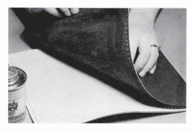
STEP 3. Apply coat of Rubber Cement to rough side of bag front and to back side of front lining (lining without pocket). Allow cement to dry until tacky. Carefully aligning holes, adhere lining to bag front with rough sides together.
