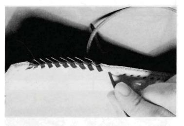
STEP 10. Beginning in second hole from edge on the left side of the bag front, lace top edge of bag front with a Double Loop Stitch. Lace across top stopping in next to last hole from edge. Do not tie off or trim lace.
