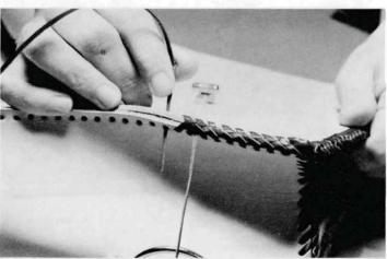
STEP 11. When lacing gusset/pocket assembly to bag front, be sure zipper is closed. Zipper pull should be to left side of the gusset/pocket assembly. Align lacing holes in right side of bag front with lacing holes in right end of gusset/pocket assembly. Continue lacing by lacing through the last hole in top of bag front and first hole of gusset twice to secure the corner. Lace around gusset and bag side until you reach next to last hole in gusset and bag side. Do not tie off or trim lace.
