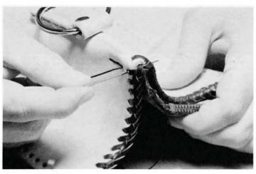
STEP 9. Fold wide end of gusset around one end of the zippered pocket, aligning the 4 holes in the end of the pocket with both sets of holes in top of gusset. Beginning in lacing hole which was previously used for Double Loop Stitch at the top of the wide end of the gusset, Using 24" of waxed thread, stitch pocket into gusset using stitching instructions in Step 7. Repeat for other side.
