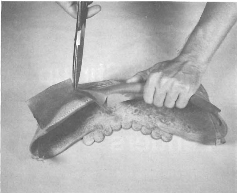
Step 16. Roll under to flesh side of fork cover making a small tight roll. Edge of roll may have to be cut so it will lie flat with no wrinkles. Cautions: do not clip edge too far or it will show after fork cover is installed.
