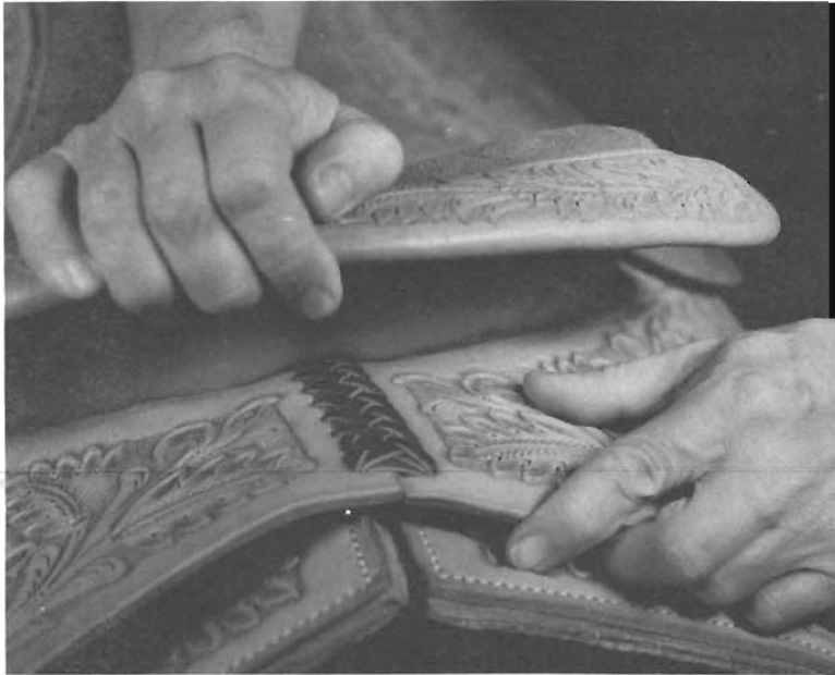
Step 61. Dampen inside edge of back jockey on flesh side. Push center of back jockey tightly up against back of cantle.
