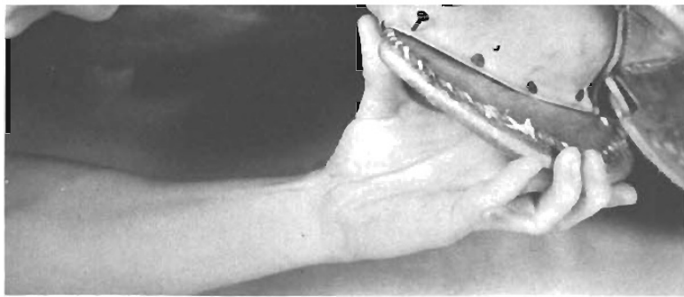
Step 29. Pull leather at base of back cantle down firmly and tack into place.
