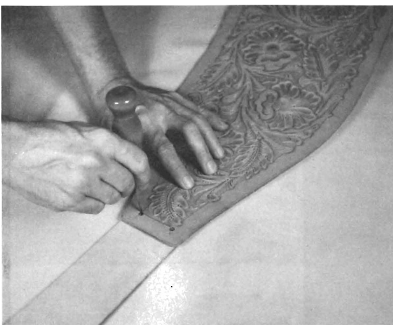
Step 40. With fender still folded mark location of holes on stirrup leather (grain side). Punch holes with no. 5 punch.
