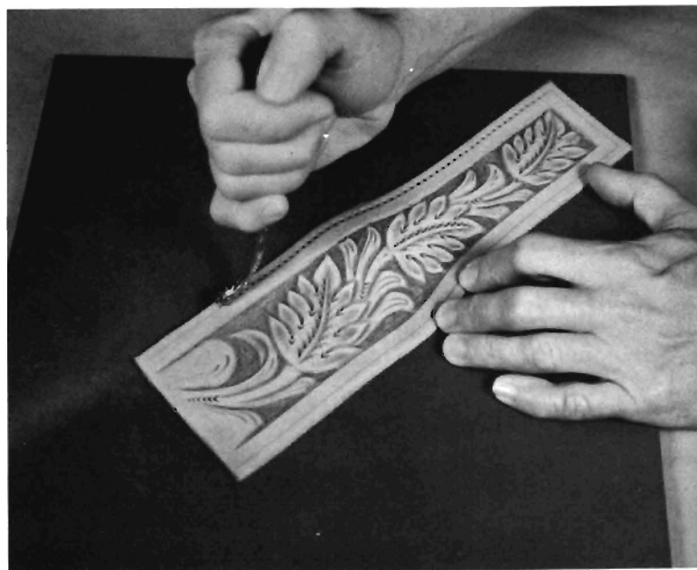
Step 84. With #5 Craftool spacer or overstitch, mark stitching holes along scribed line.
