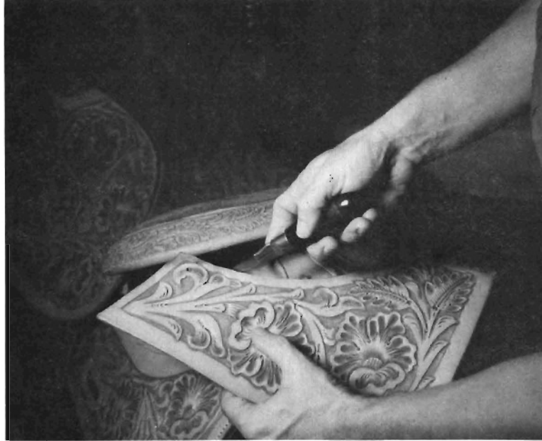
Step 64. Back jockeys should be parallel to skirts at back and side. If they are not, you may have to trim inside edge of jockeys so they may be properly aligned. When you are sure of proper alignment, pull tightly around base of cantle (so lace centers properly in back) and tack as you did on other side.
