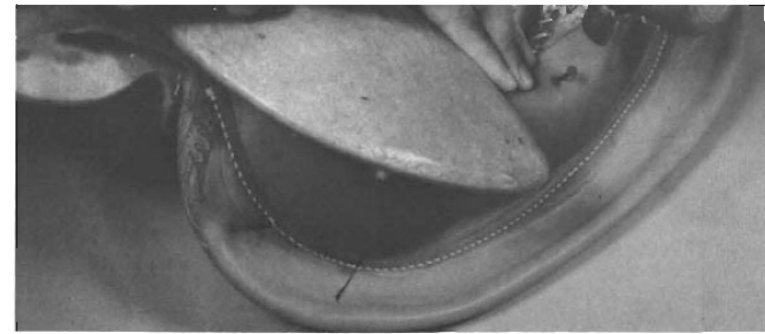
Step 28. Pull leather (on back cantle) tightly and firmly under cantle and tack into place. Using 1/8" tacks.
