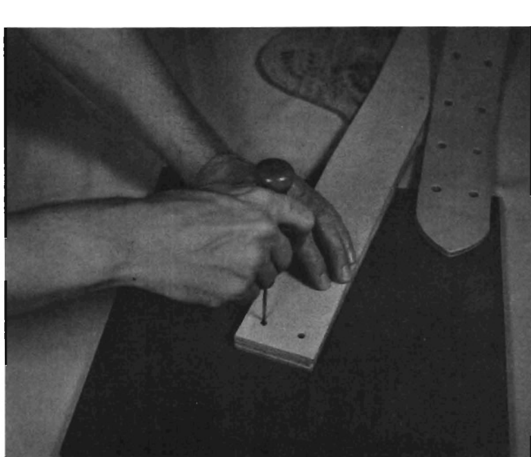
Step 34. Place the stirrup end of left fender (flesh side up) underneath end of stirrup leather, aligning ends and edges. Mark the two rivet holes and punch with no. 5 punch.
