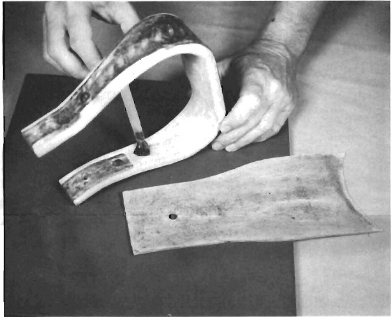
Step 78. Apply Craftsman cement to inside of stirrup.
