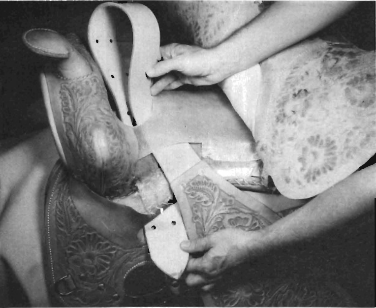
Step 54. Bring leather around bar and back between bar and skirt. Install fender and stirrup leather on other side.
