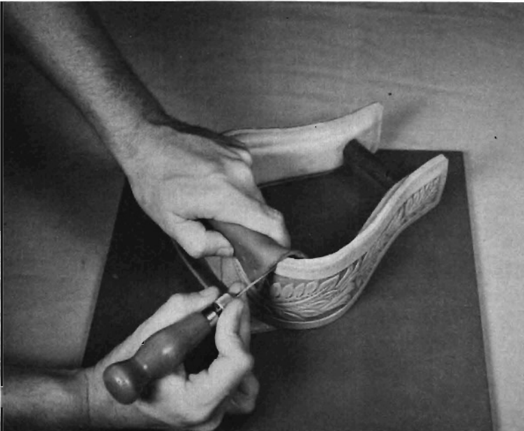
Step 89. Dampen thread cover, center, and form around bottom of stirrup. With awl, mark (on bottom of stirrup) 4 points where tread cover wraps around edges of stirrup bottom.
