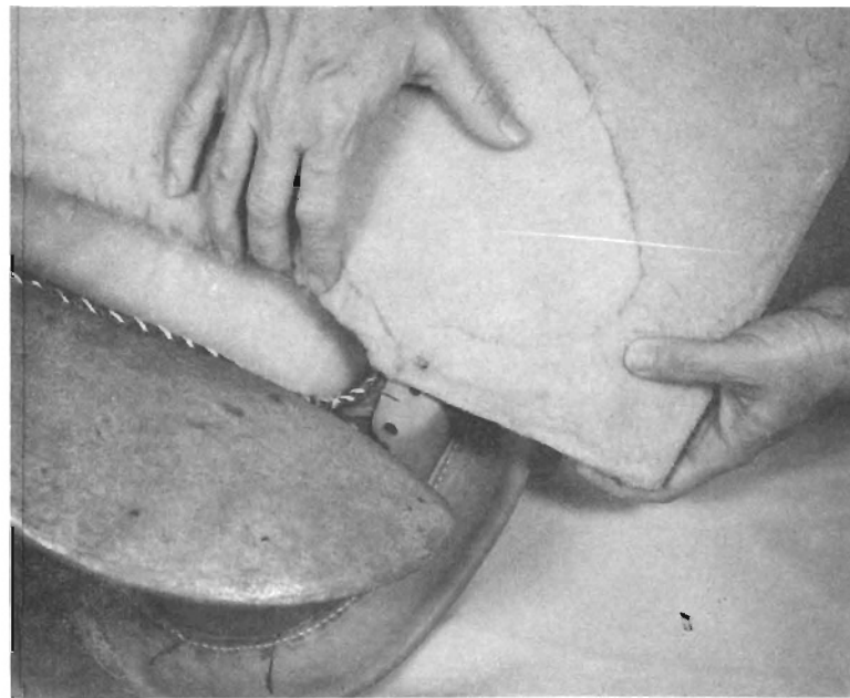
Step 47. Place top back edge of skirt in center and nail through skirt and into bottom of cantle. This completes proper alignment of one skirt. Install other skirt in same manner.
