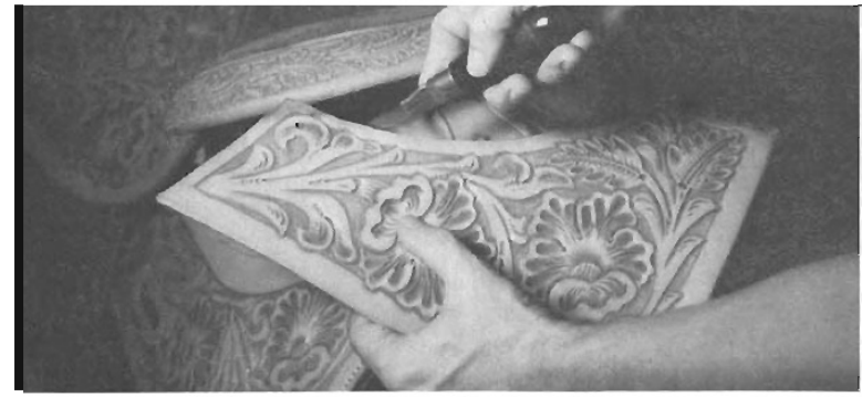
Step 64. Back jockeys should be parallel to skirts at back and side. If they are not, you may have to trim inside edge of jockeys so they may be properly aligned. When you are sure of proper alignment, pull tightly around base of cantle (so lace centers properly in back) and tack as you did on other side.
