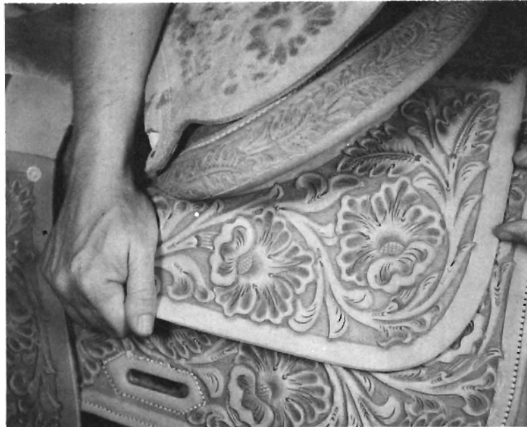
Step 63. On opposite side pull back jockey tightly around back of cantle.
