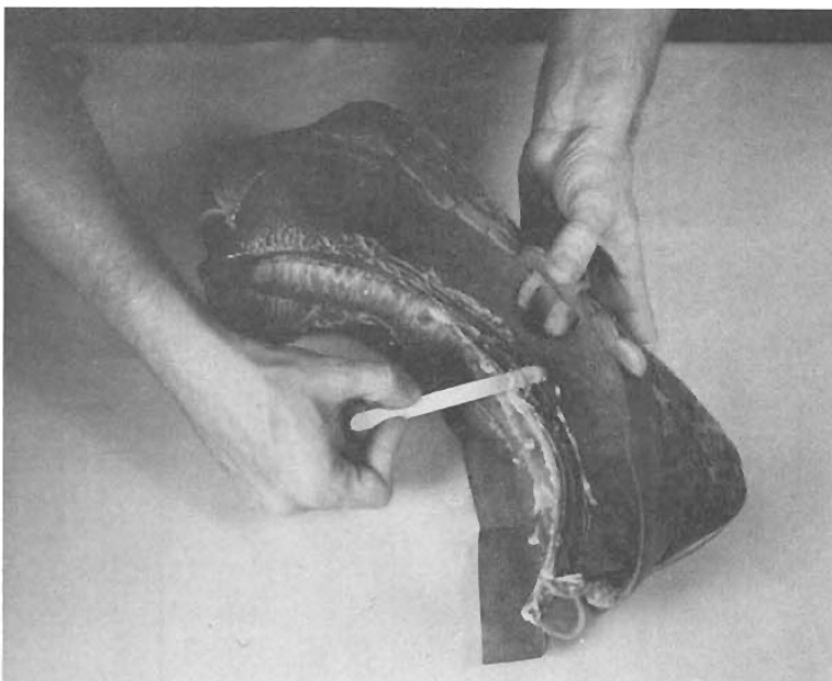
Step 17. After you have fitted binder apply paste to flesh side of binder and roll into place smoothing out all wrinkles.
