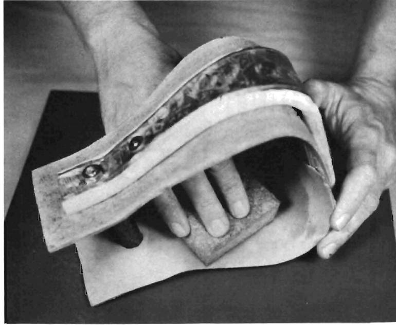
Step 81. Dampen stirrup linings.
