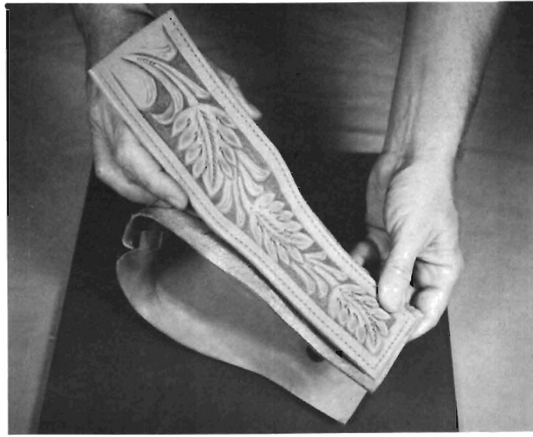
Step 85. Apply Craftsman cement to stirrup covers and outside of stirrup. Centering stirrup covers on stirrup (leaving 3/8" of stirrup cover above top of stirrup) begin sticking cover and lining together at edges.
