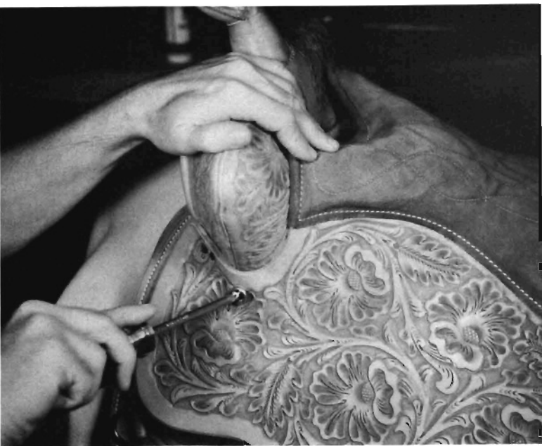
Step 70. Drill hole (1/8" drill bit) 3/4" from edge of jockey and just behind side seam. Install 1 1/2" screw and washer.
