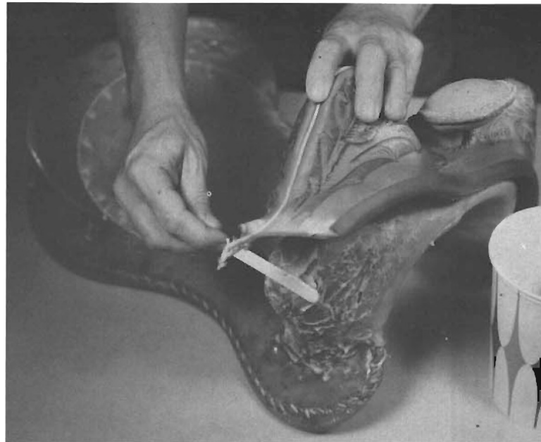
Step 20. Holding corners of fork cover up, apply paste liberally to swells and fork area, especially to point of swells. This will fill area around swells so they will be smooth and firm.
