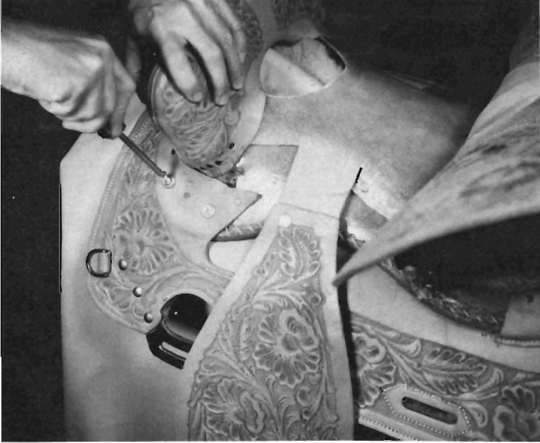
Step 59. Drill and place 2-1" screws as shown, on each side.
