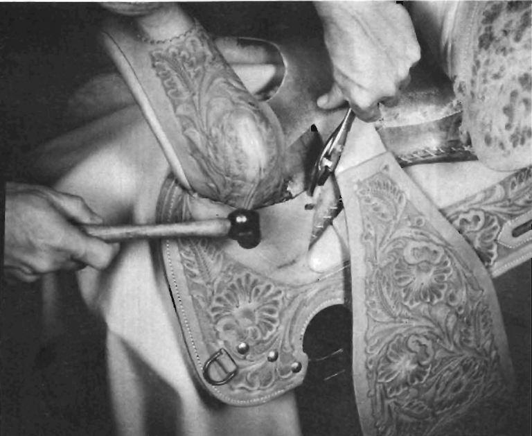
Step 57. To secure front bars in front bar pocket, pull (with pliers or saddle awl) leather tightly around fork and tack with 7/8" tack.
