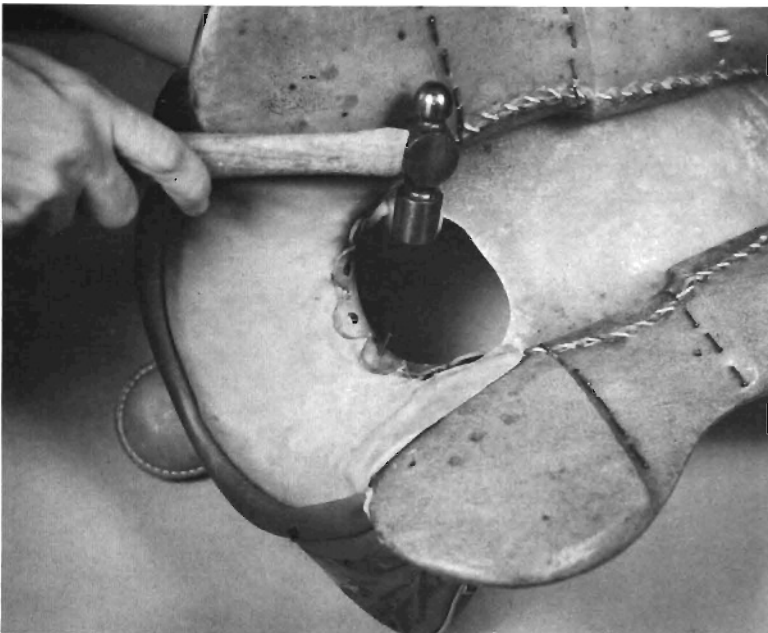
Step 23. Pull scalloped end of fork cover tightly under tree to gullet and tack.
