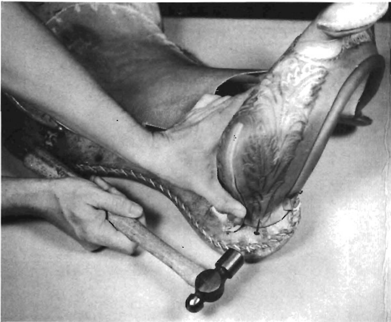
Step 22. After pulling fork cover as smooth and tight against tree as possible, drive first tack (1 1/8" long) close to side seam at base of fork cover. Be sure tacks are low enough so they will be hidden. Drive second tack at front, at base of binder. Drive third tack between first and second at base of fork cover. Drive 3 tacks in similar manner behind side seam. Secure other side of fork cover in same manner.
