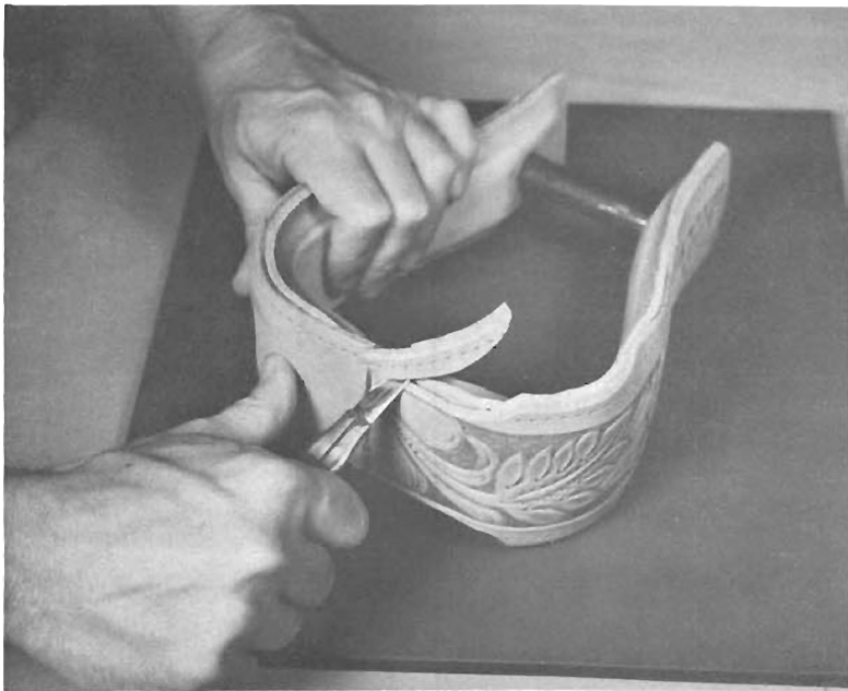
Step 90. Between the points you have marked on stirrup bottom, trim cover and lining off next to edge of stirrup.
