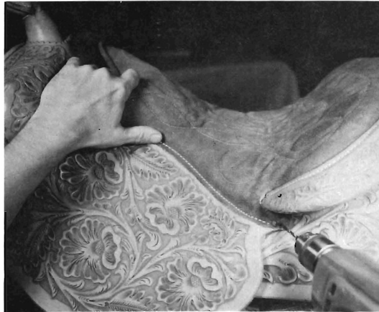
Step 67. Drill (with 1/8" bit) hole where center of rosette was marked. Mark and drill hole on opposite side also.
