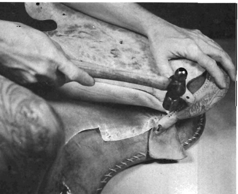
Step 30. Pull ends of cantle binder forward (with pliers or saddlers awl) and tack into place (use 2-1 1/8" tacks) on bar at the base of cantle. Be sure seat is centered.
