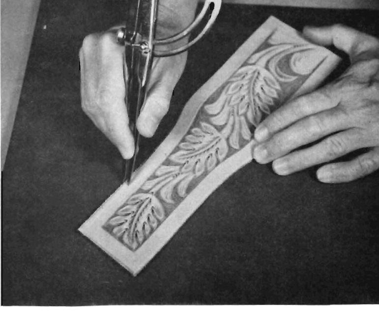
Step 83. Scribe line 1/4" from edge around sides and top of 2 stirrup covers.
