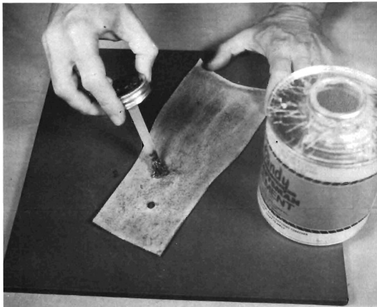
Step 77. Apply contact type cement (Craftsman) to flesh side of stirrup lining. (Apply cement to both halves.)
