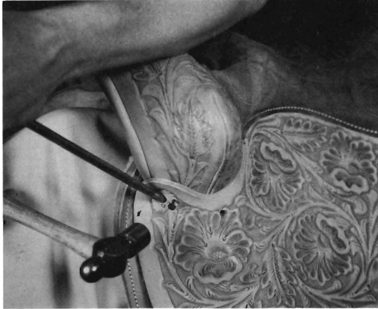
Step 69. With saddlers awl, pull front jockey tightly around base of fork and drive (1 1/8") tack to hold in place. Tack opposite side.
