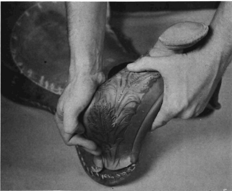
Step 21. Pull both sides of fork cover down over tree and smooth into place so there are no wrinkles. Use your hand to smooth leather into place or use saddlers awl (or phillips head screwdriver) to drive in at base of cover and pull into place.
