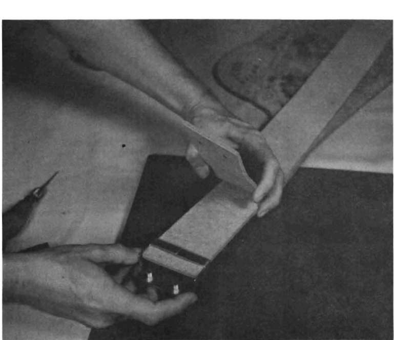
Step 35. Slip tongue end of stirrup buckle on fender (stirrup end) as shown. Push buckle up about 8", out of way.
