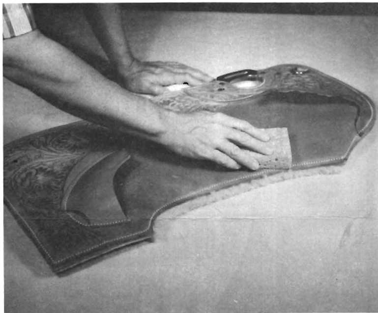
Step 42. Dampen front and back bar pockets and area on skirt between these pockets.
