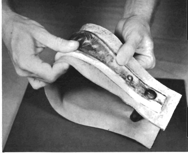
Step 82. With fingers, form stirrup linings around sides of stirrup.
