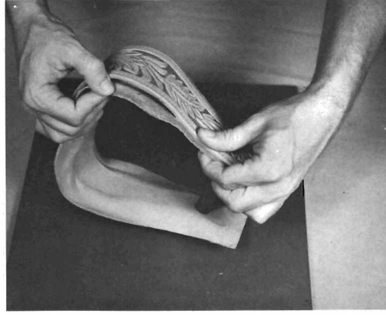
Step 86. Stirrup cover will remain flat and lining is brought around stirrup to meet cover. Trim cover off at bottom if 2 halves overlap.
