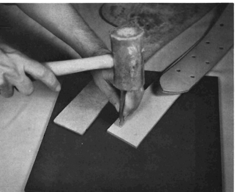
Step 33. Punch rivet holes with #5 punch.
