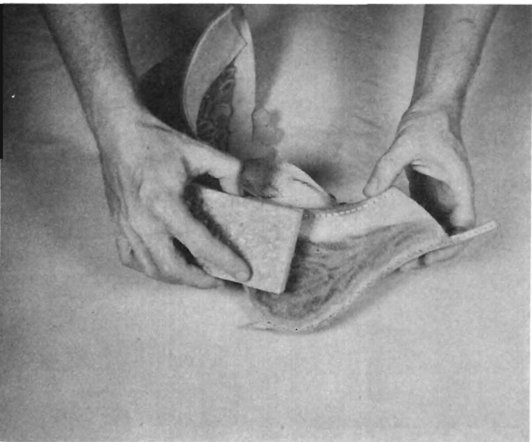
Step 11. Dampen flesh side of fork cover with sponge before turning grain side out. Do not apply so much moisture that it soaks through to grain side.
