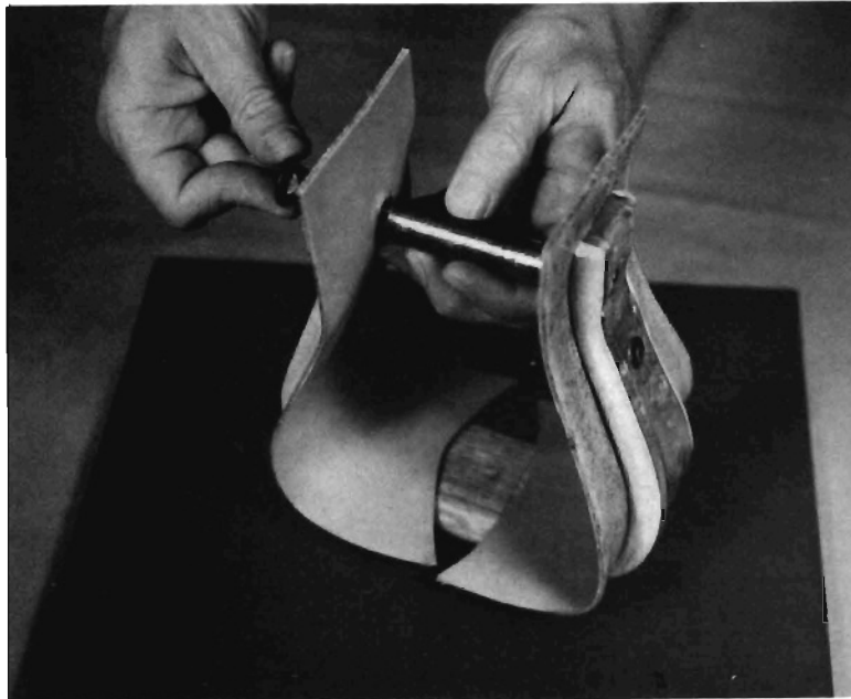
Step 80. Install bolt, roller and nut on stirrup. Saw or grind end of bolt off even with nut.
