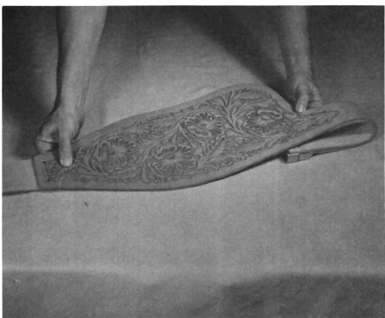
Step 39. Fold stirrup end of fender (with stirrup leather and buckle attached) under as shown.
