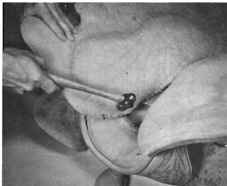
Step 50. Secure top front of skirt with 2 nails driven through skirt into gullet. Secure both sides.
