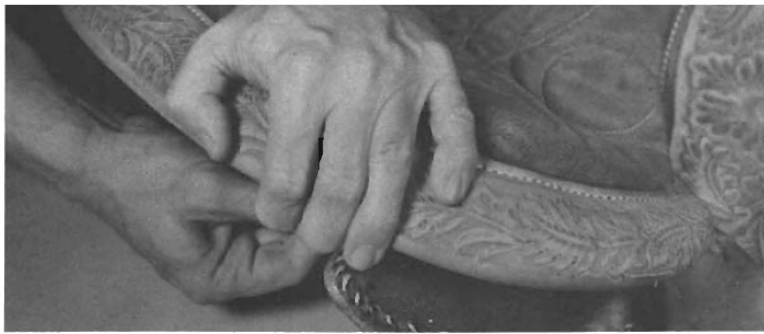
Step 27. Push seat firmly against cantle smoothing leather tightly under "dish" of cantle.
