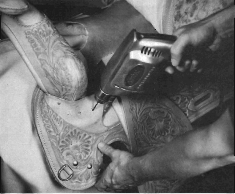
Step 58. Place 2 more tacks as shown. Tack other side in same manner. Using 1/8" bit, drill hole through leather and into bar.
