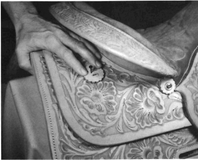
Step 74. On back jockey, center large rosette with 2 slots (grain side up) 4 1/4" from center of lacing and 3 1/4" from back edge of jockey. Drive (1 1/8") tack through leather and into bar to hold rosette in place.
