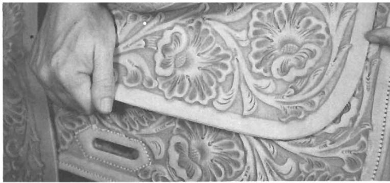
Step 63. On opposite side pull back jockey tightly around back of cantle.
