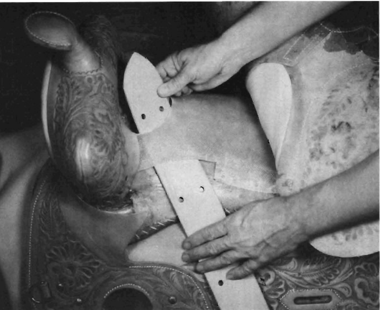
Step 53. Insert pointed end of stirrup leather (grain side up) between ground seat and bar.
