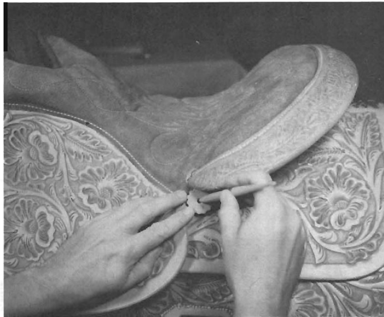
Step 66. Place leather rosette on "ear" and mark center. Rosette should cover tack and secure "ear" on side jockey.
