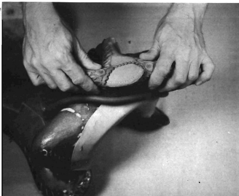
Step 19. Lightly dampen grain side of fork cover. Using a side to side motion pull fork cover over horn.
