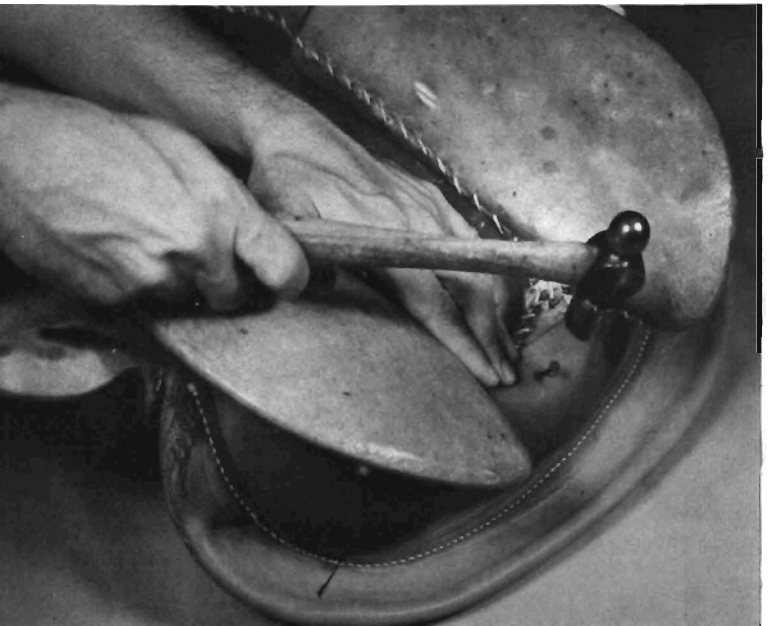
Step 28. Pull leather (on back cantle) tightly and firmly under cantle and tack into place. Using 1/8" tacks.
