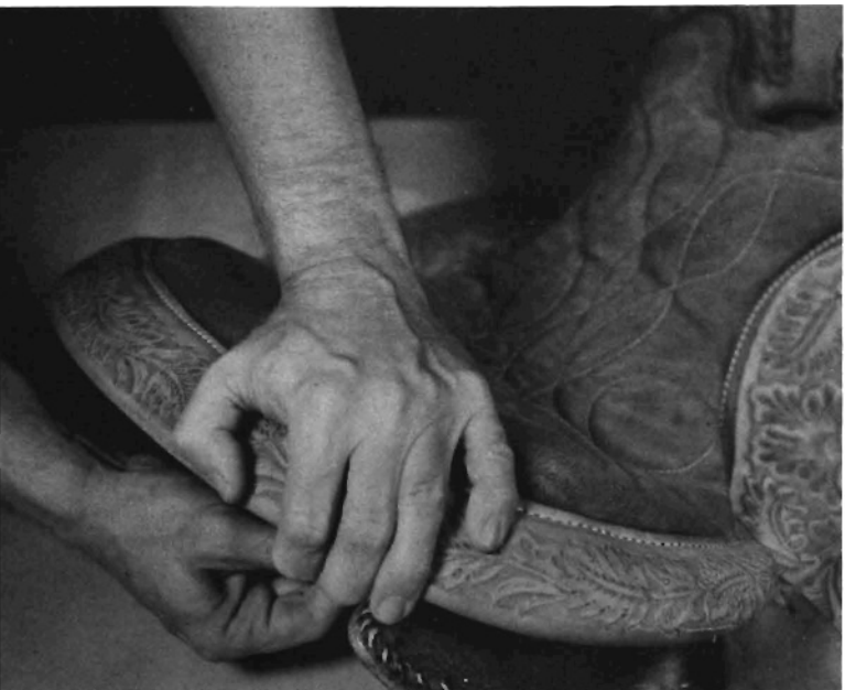
Step 27. Push seat firmly against cantle smoothing leather tightly under "dish" of cantle.
