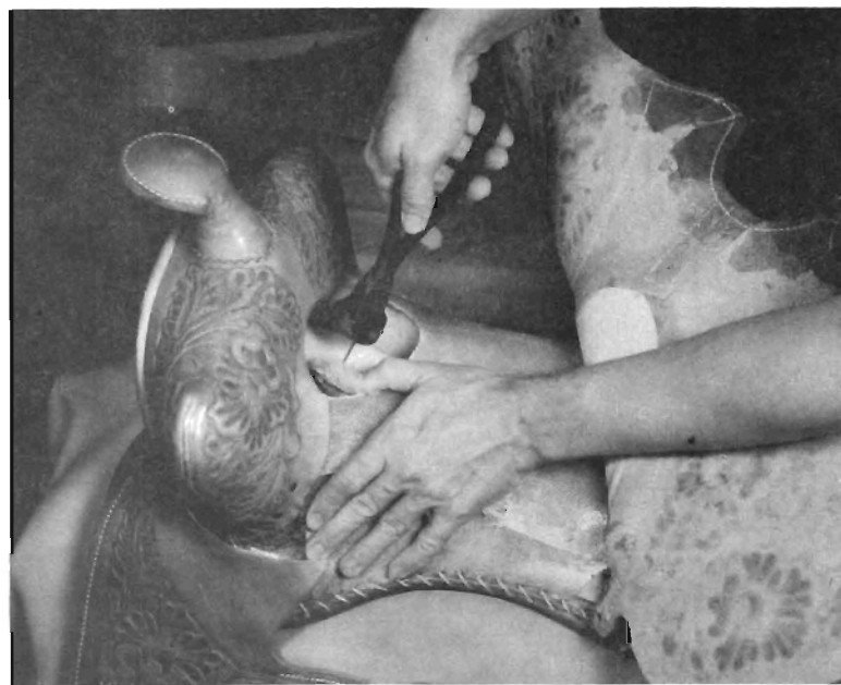
Step 52. Remove temporary nails in points at front of skirts (step 45). This will make installing fenders and stirrup leathers easier.
