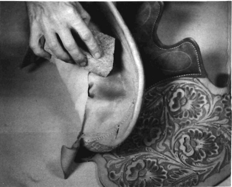
Step 24. Thoroughly dampen back of seat.
