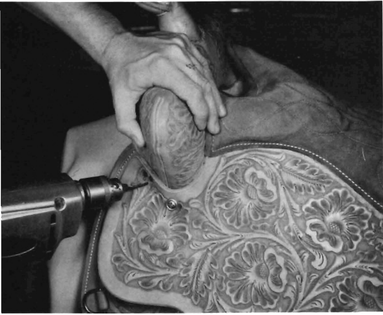
Step 71. Drill hole (1/8" drill bit) just below tack, in front jockey.
