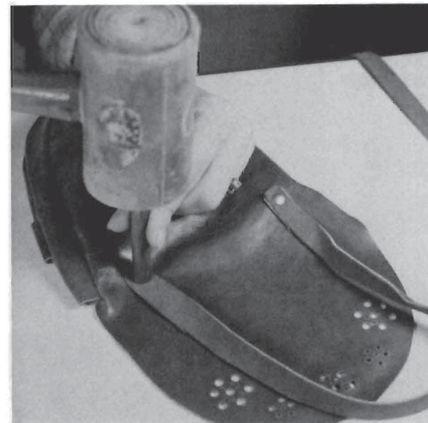
STEP 7. Take rivet stud and push it through one hole in bag back from inside bag. Now push hole in one strap over rivet stud on outside of bag back. Place cap of rivet over stud. Put the whole assembly on a solid surface. Place rivet setter on rivet cap and set rivet by striking setter sharply with a mallet. Repeat with other strap on other side of bag back.
