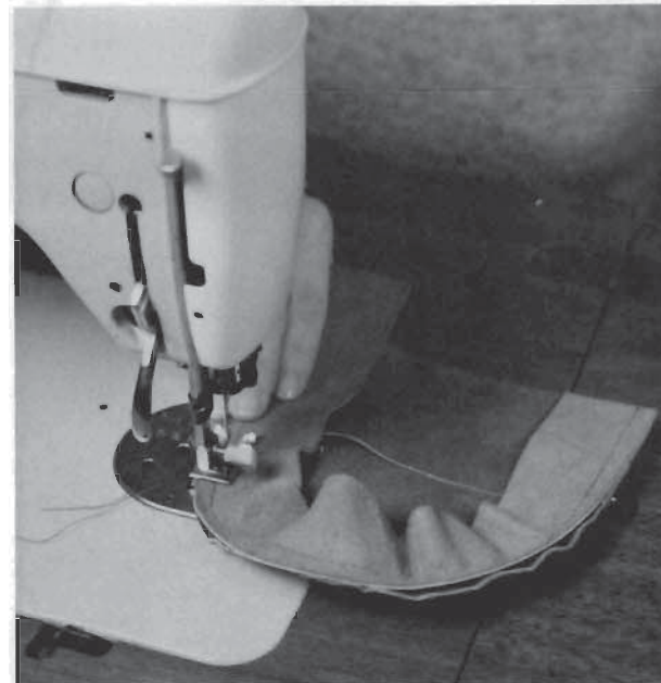
STEP 4. Align one edge of gusset with edge of bag front, grain sides together, and stitch gusset in place, being sure to catch ends of front strap in seam.
