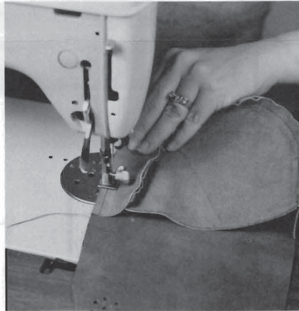
STEP 5. Align other edge of gusset with edges of bag back, grain sides together, and stitch gusset in place.
