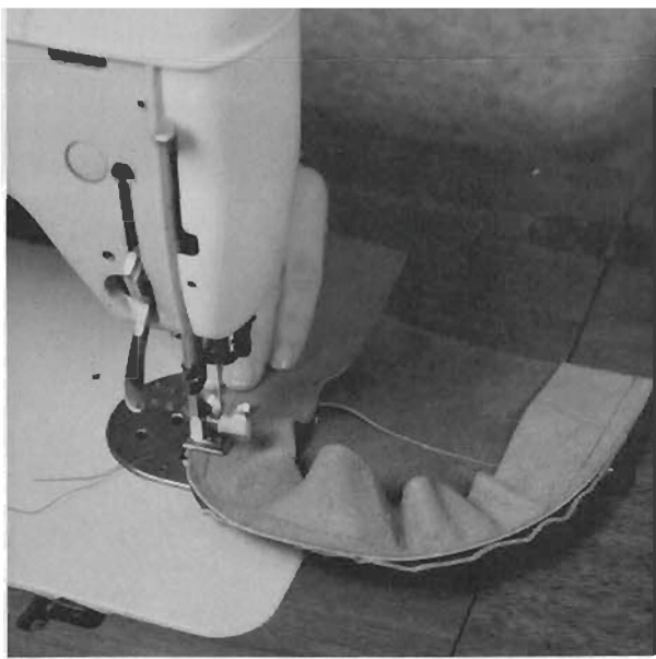
STEP 4. Align one edge of gusset with edge of bag front, grain sides together, and stitch gusset in place, being sure to catch ends of front strap in seam.
