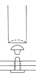
For best results use a rivet setter and rawhide mallet Use rivet slightly longer than thickness of leathers.
