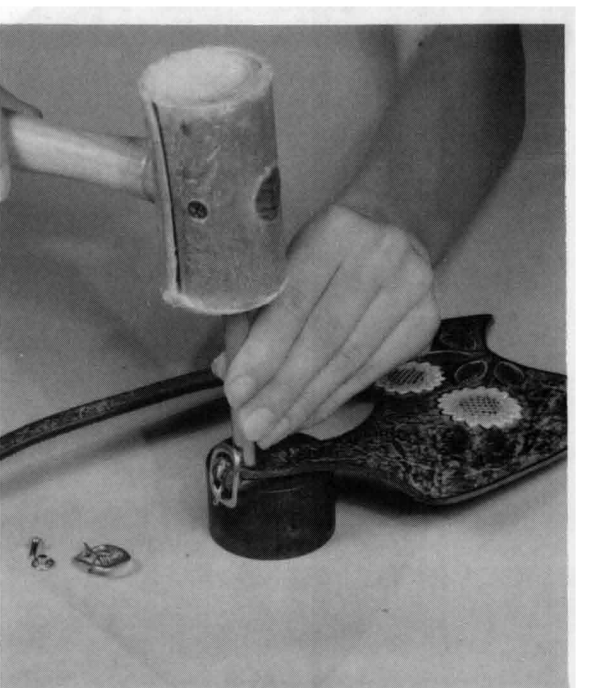
STEP 7: Insert buckle tongue through slits from grain side of buckle strap; then fold buckle strap around buckle (grain side to grain side) and align rivet holes. Set rapid rivets using rapid rivet instructions on reverse side of sheet. Punch holes in other strap as indicated on pattern.
