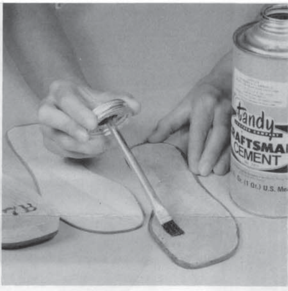
STEP 5: Apply Craftsman Cement to the top of the wooden soles and to flesh side of the leather soles. Allow to dry until it becomes tacky.
